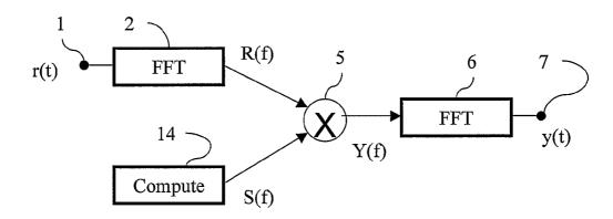
(57) Abstract: A signal is filtered by multiplying its Fourier transform by the Fourier transform of a reference sequence to which the filtering is to be matched. The reference sequence (e.g. a Golay sequence pair) is defined as an iterative combination of shorter sequences and its Fourier transform is generated by an iterative process of combining the Fourier transforms of a shorter starting sequence.
