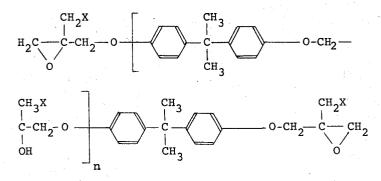
Wherein *n* is 0 to 3 and X is hydrogen or chlorine. The epoxy resin (3) is prepared by condensation of  $\beta$ -methyl epichlorohydrin or  $\beta$ -chloromethyl epichlo-<sup>20</sup> rohydrin with bisphenol-A. The preparation process is disclosed in, for example, U.S. Pat. No. 3,553,165 (Patented on Jan. 5, 1971 by Chiyoda Kako Kensetsu Kabushiki Kaisha).
