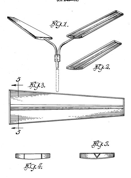
FIG. 1 is a perspective view of an outdoor lighting fixture, showing my new design with the standard shown broken away in part to indicate indeterminate length;
