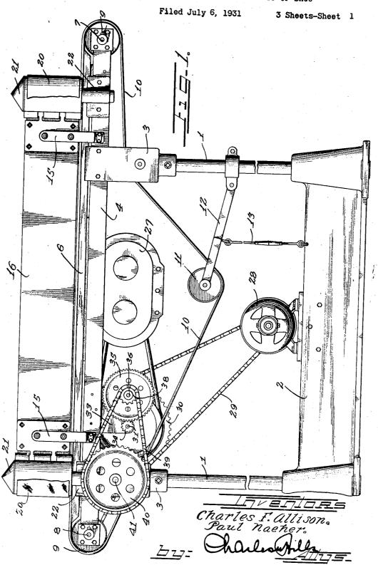
VIBRATING MACHINE FOR SETTLING CONTENTS OF BAGS
