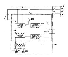
control circuit which generates a clock signal including pulses with a predetermined period. The sensing circuit determines the current or the temperature of the sensing element during an active period of the clock signal.
