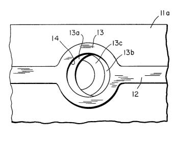
ings in the first and second aligned land areas; and plating the hole to provide an electrically conductive via.
