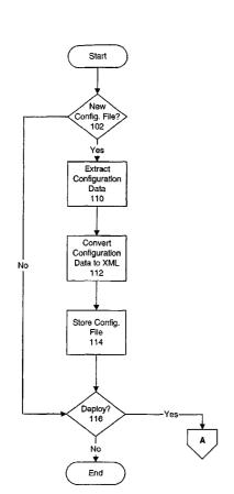
(57) Abstract: Multiple devices within a data communication network can be configured according to a single configuration profile. Configuration profile data is stored in a configuration file. Connections are made to individual devices, and the data in the configuration file is transformed into device-specific commands.
