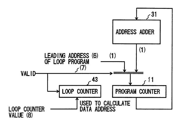
VALID: INDICATE LOOP PROGRAM TO BE EXECUTED. WHEN VALID IS ACTIVE, SELECTOR SELECTS LOOP ADDRESS AND WRITING INTO REGISTER INDICATING LOOP NUMBER IS PERFORMED.
