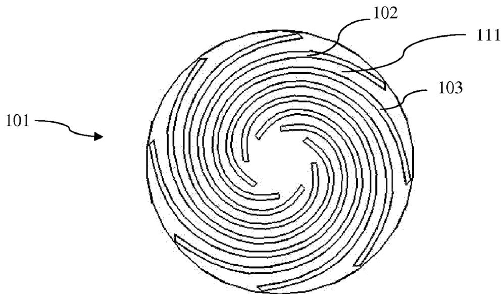
**FIG. 1** A radial pattern of heat exchange channels
