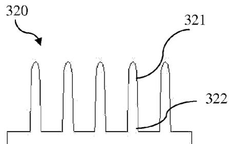
FIG. 3.2 Guide fins with rounded
