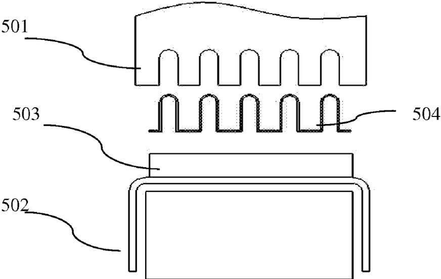
FIG 5.1 Impact Bond Extrusion Process
