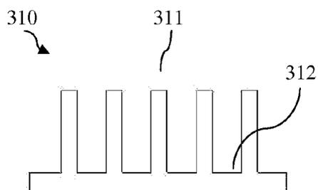
FIG. 3.1 Guide fins with flat top
