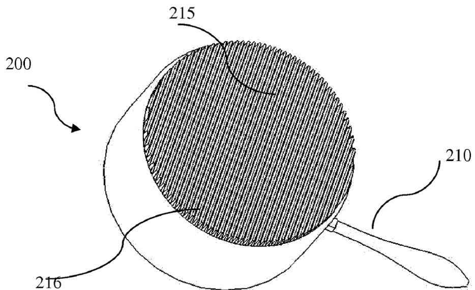
**FIG. 2** A piece of cookware with linear pattern of channels
