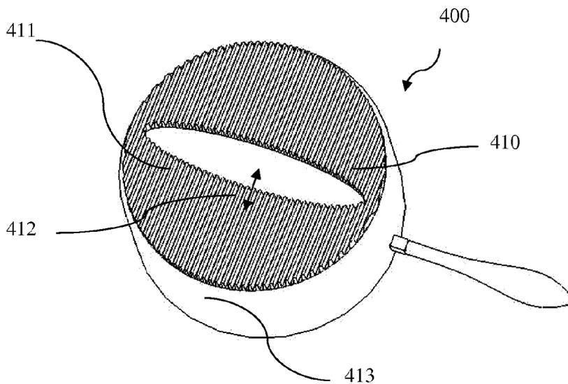
FIG. 4 A piece of cookware with an elliptical entrance opening in exchange channels
