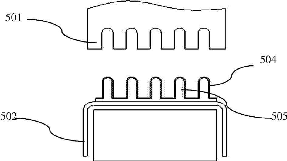
FIG 5.2 Impact Bond Extrusion Process
