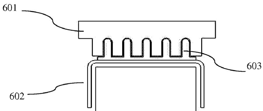
**FIG. 6.2** Removable punch with pot assembly
