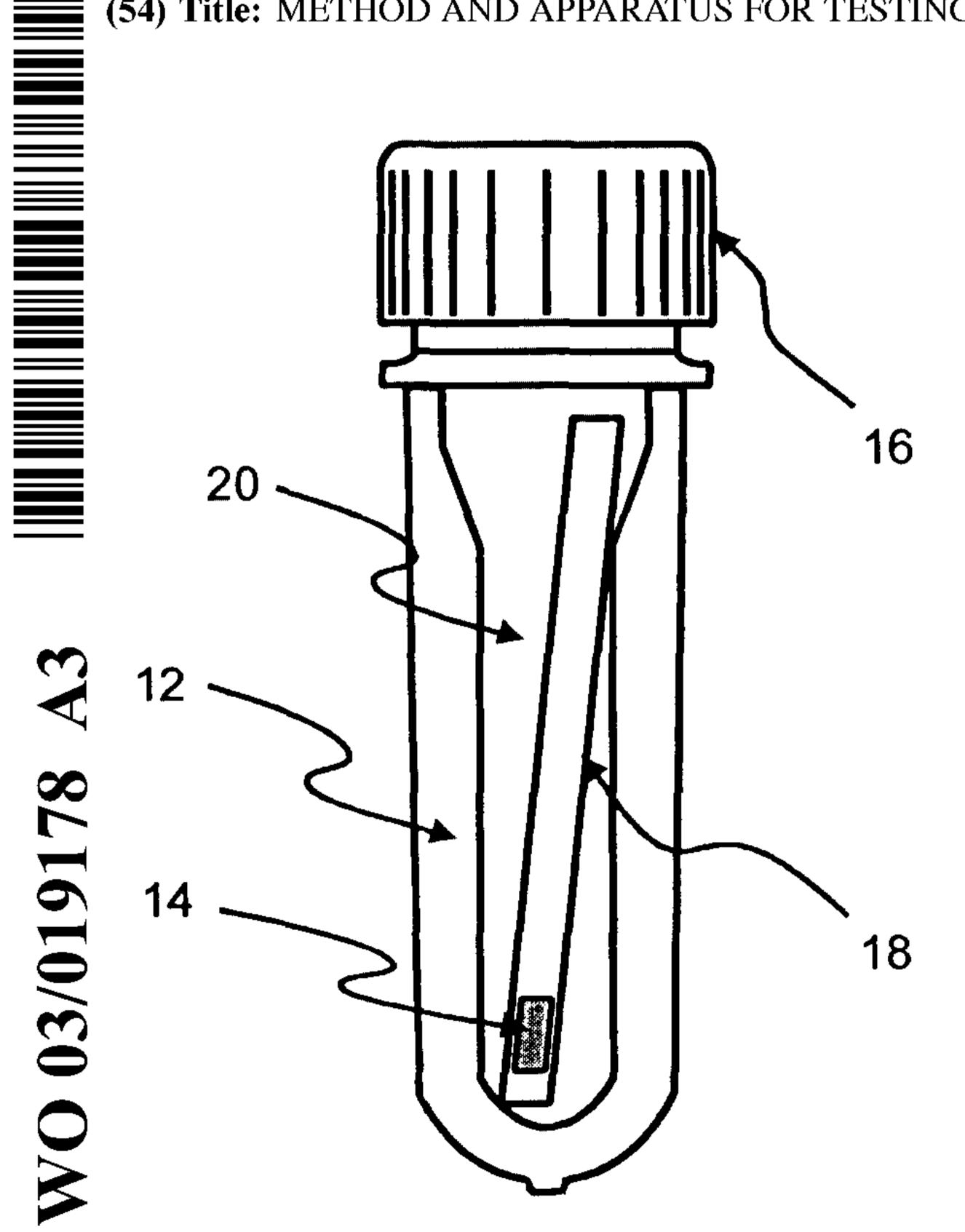
(57) Abstract: A test strip, methods for making and using the test strip, and a kit are described, which allow for the simple and efficient determination of the acetaldehyde content in a polyester polymer. The strip and methods have application, for example, in the manufacture of polyethylene terephthalate preforms and containers, where existing methods for testing for acetaldehyde are cumbersome and time consuming.
