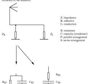
The above presented scheme describes the basic situation. ( $R_{KS}$  represents: resistance (R) caused by the adhesive, in a series arrangement as model).
