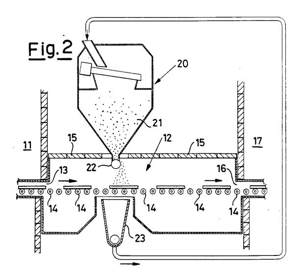
"PROCESS AND APPARATUS FOR PRODUCING GLAZED CERAMIC TILES, AND TILES SO OBTAINED"
