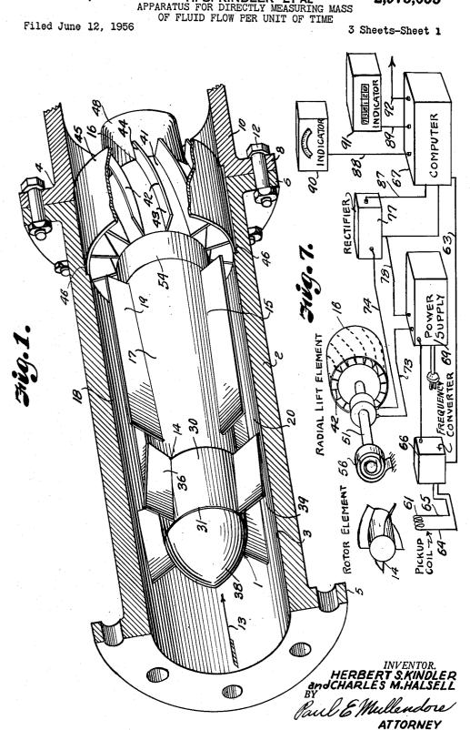
March 21, 1961 2,975,635 H. S. KINDLER ET AL APPARATUS FOR DIRECTLY MEASURING MASS OF FLUID FLOW PER UNIT OF TIME
