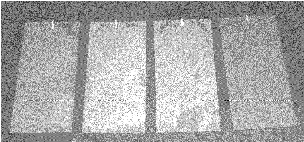
Reverse side salt fog results after 2 weeks
