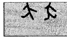
Stress corrosion cracking
