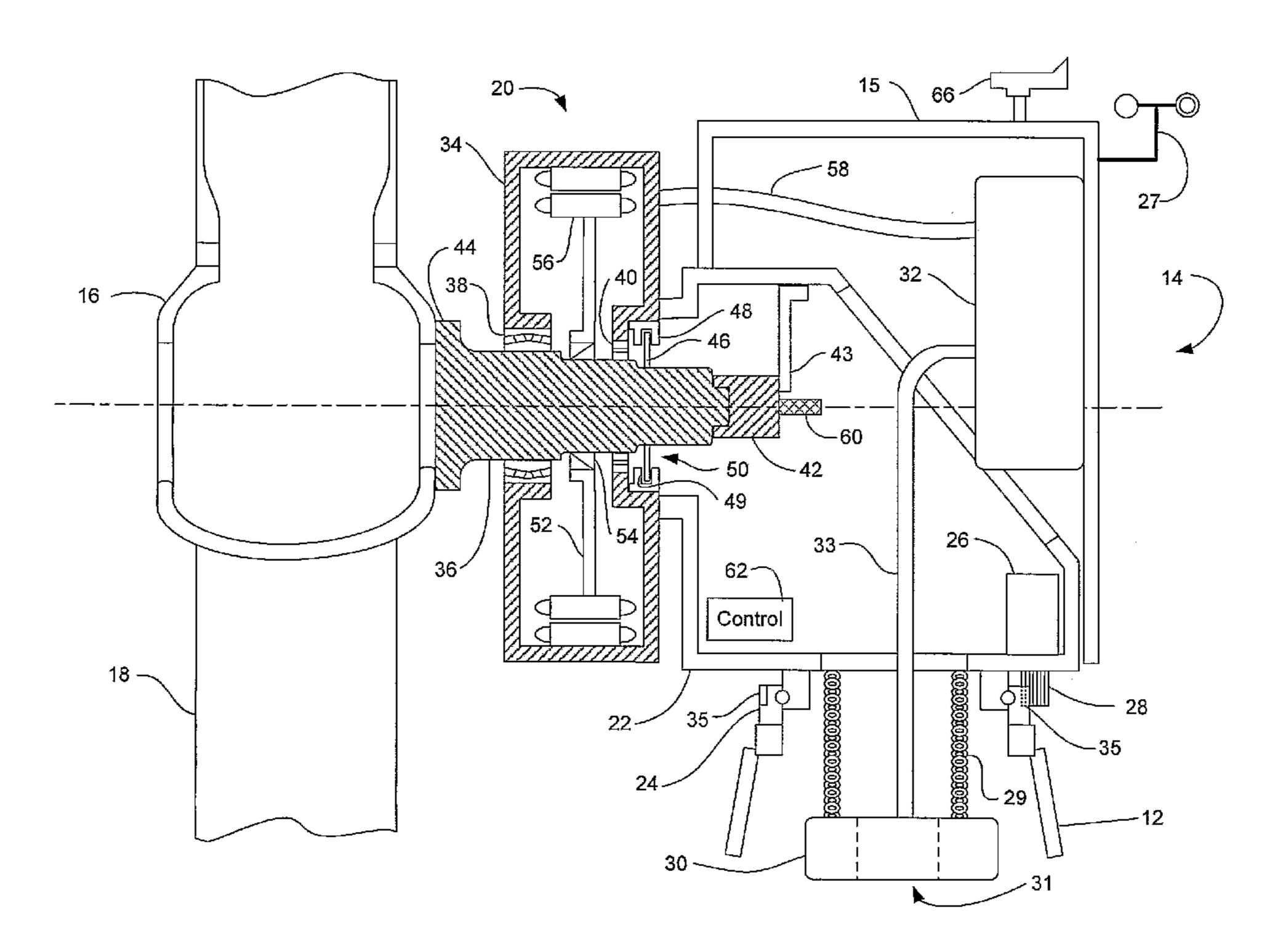
(57) Abstract: A wind turbine is provided that minimizes the size of the drive train and nacelle while maintaining the power electronics and transformer at the top of the tower. The turbine includes a direct drive generator having an integrated disk brake positioned radially inside the stator while minimizing the potential for contamination. The turbine further includes a means for mounting a transformer below the nacelle within the tower.
