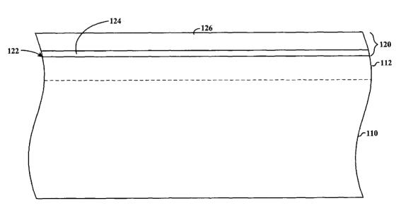
process is implemented to grow Germanium (Ge) containing material, such as heteroepitaxial-Germanium, on a substrate including Silicon (Si) or Silicon-containing material. In certain applications, defects are generally confined near a Silicon/Germanium interface, with defect threading to an upper surface of the Germanium containing material generally being inhibited. These approaches are applicable to a variety of devices including Germanium MOS capacitors, pMOSFETs and optoelectronic devices.
