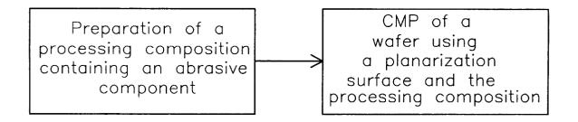
Planarization Using a Processing Composition Containing an Abrasive Component
