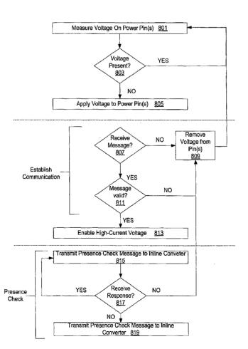
(57) Abstract: A system, method, and apparatus for inline audio/visual conversion are described. Power to an inline converter is provided over the A/V cable that couples the converter to a destination such as a selector.
