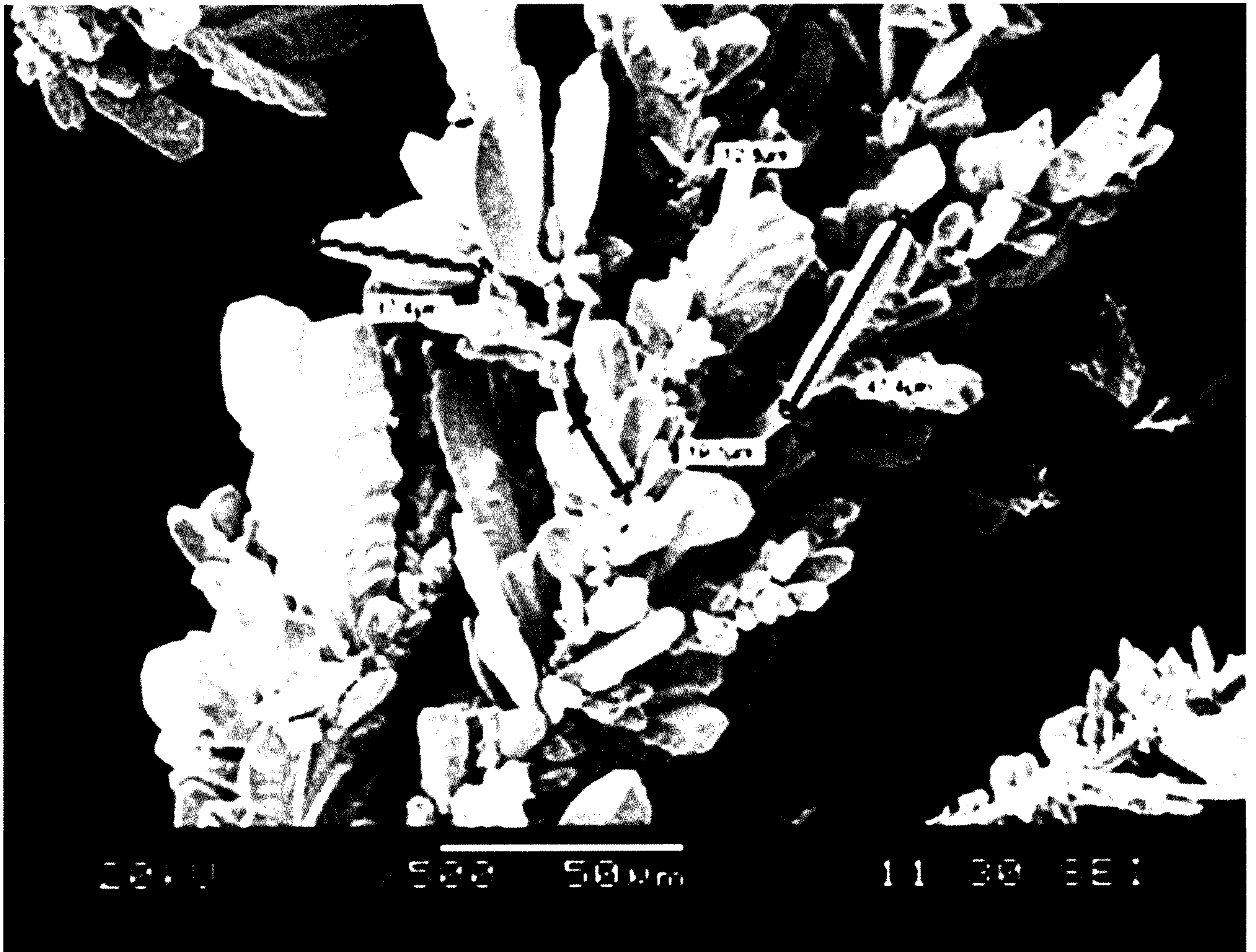
SEM image of deposited copper powder
