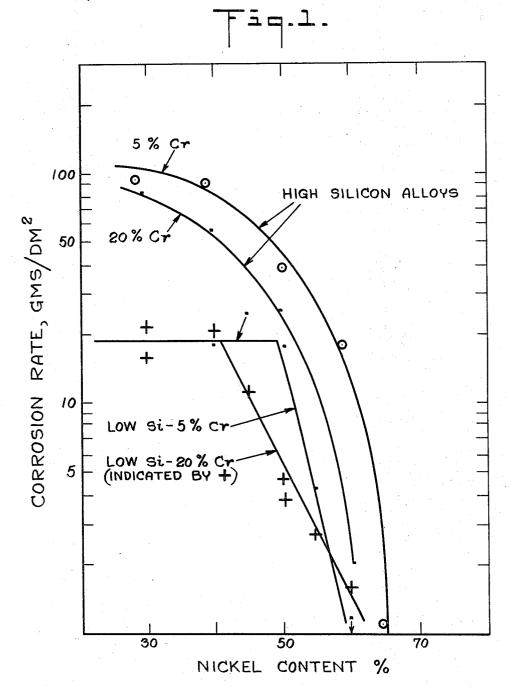
CORROSION RATES OF SIMPLE FE-CR-NI ALLOYS AS A FUNCTION OF NI, CR AND SI.
