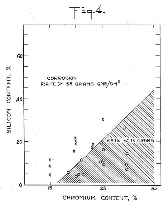
RELATIONSHIP OF CHROMIUM AND SILICON CONTENTS ON CORROSION BEHAVIOR OF FE-NI-CR-MN ALLOYS CONTAING TITANIUM AND ALUMINUM.
