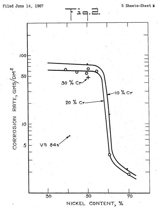
CORROSION RATES OF LOW SILICON FE-CR-NI ALLOYS CONTAINING TITANIUM AND ALUMINUM
