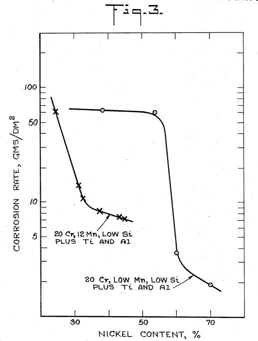
EFFECT OF 12 MN ON CRITICAL NICKEL CONTENT OF NI-FE-CR ALLOYS HARDENED WITH TI AND A1
