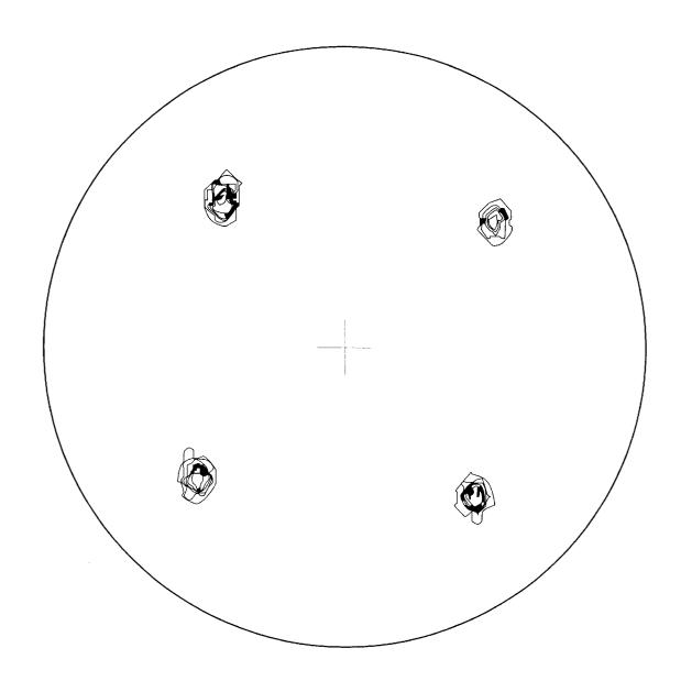
Ni-13at%Cr-0.03at%Mg alloy Annealing Temperature = 1200°C
