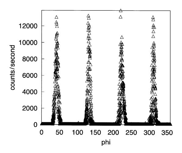
Ni-9at%W alloy Annealing Temperature = 1200°C
