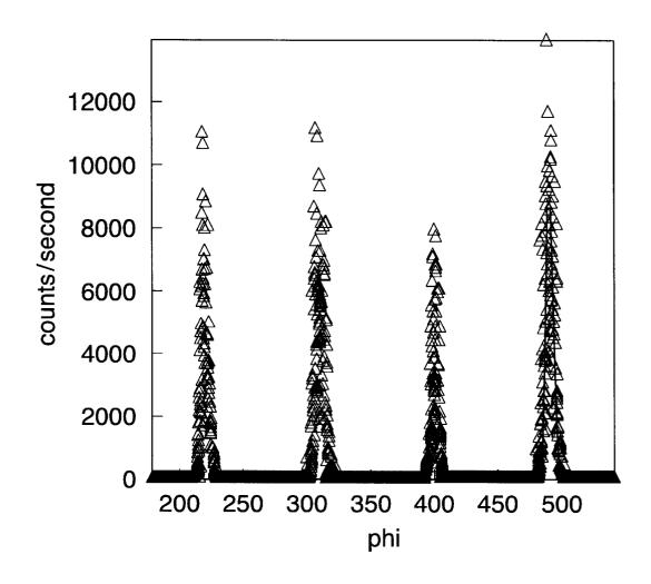
Ni-13at%Cr-0.03at%Mg alloy Annealing Temperature = 1400°C
