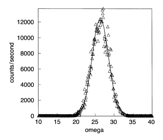
Ni-13at%Cr-0.03at%Mg alloy Annealing Temperature = 1200°C
