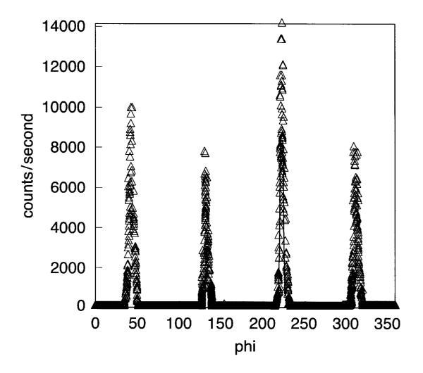
Ni-9at%W alloy Annealing Temperature = 1400°C
