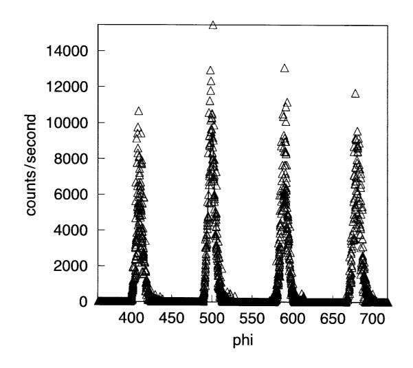
Ni-9at%W-0.03at%Mg alloy Annealing Temperature = 1200°C
