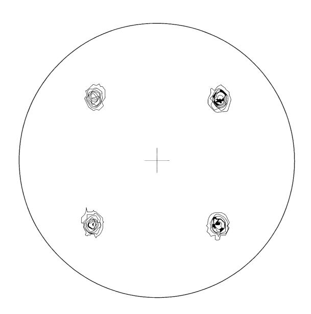
Ni-9at%W-0.03at%Mg alloy Annealing Temperature = 1200°C
