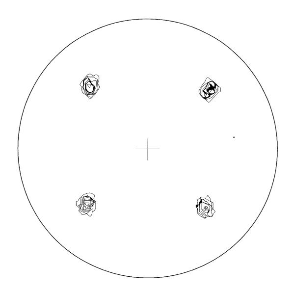
Ni-0.03at%Mg alloy Annealing Temperature = 1200°C
