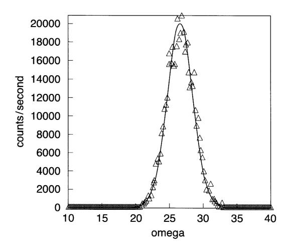
Ni-13at%Cr alloy Annealing Temperature = 1400°C
