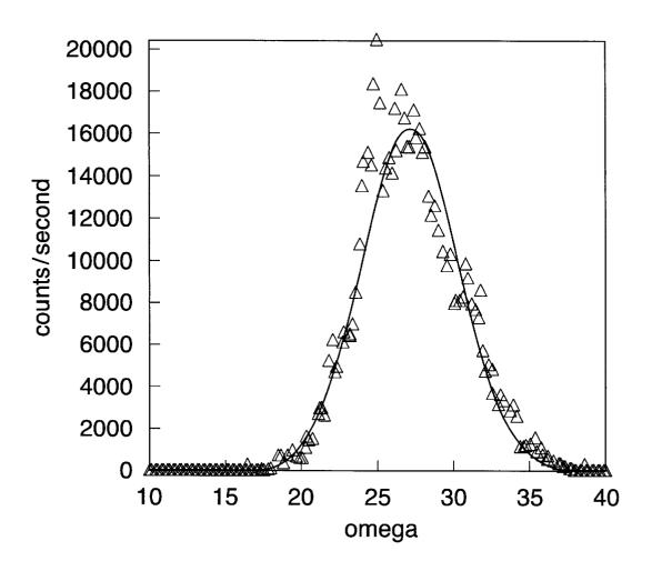
Ni-9at%W-0.03at%Mg alloy Annealing Temperature = 1400°C
