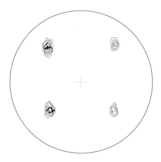
Ni-13at%Cr alloy Annealing Temperature = 1200°C
