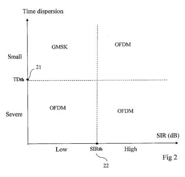
(57) Abstract: A modulation method for data packets transmitted on a mobile communication channel, the method comprising a first linear modulation mode, to be used when the radio conditions are good, and a second constant envelop modulation mode, to be used when the radio conditions are poor. Since a constant envelope-modulated signal is degraded more when time dispersion occurs, the first linear modulation mode is also used when the time dispersion is severe.
