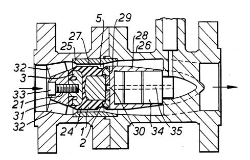
VALVE ASSEMBLY FOR CONTROLLING FLUID
