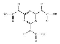
**[0115]** Examples of especially suitable tris(alkoxycarbonylamino)triazines are described in the patents U.S. Pat. No. 4,939,213 A, U.S. Pat. No. 5,084,541 A, and EP 0 624 577 A1. Use is made in particular of the tris(methoxy-, tris(butoxy- and/or tris(2-ethylhexoxycarbonylamino)-triazines.
