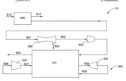
gaseous natural gas stream to obtain a second gaseous natural gas stream, and a cold box for receiving the cold stream of refrigerant and the second gaseous natural gas stream and cooling the second gaseous natural gas stream to obtain a liquefied natural gas by heat exchanging between the second gaseous natural gas stream and the cold stream of refrigerant.
