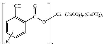
wherein R is an alkyl group derived from an isomerized alpha olefin having from about 12 to about 30 carbon atoms per molecule, having at least about 23%-98 wt % branching and a residual alpha olefin content of between at least about 9 wt % to about 30 wt %; and wherein y and z are independently whole or partial integers, and further wherein said overbased carboxylate detergent has a TBN of greater than 250.
