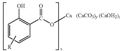
wherein R is an alkyl group derived from an isomerized alpha olefin having from about 12 to about 30 carbon atoms per molecule, having 15-98 wt % branching and a residual alpha olefin content of between from about 0.1 to about 30 wt %; and wherein y and z are independently whole or partial integers.
