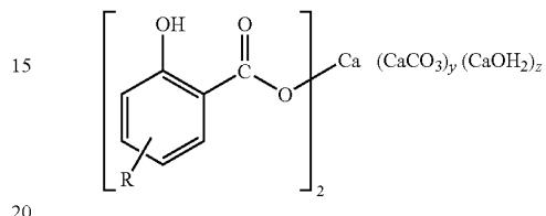
wherein R is an alkyl group derived from said isomerized alpha olefins and wherein y and z are independently whole or partial integers; and further wherein said overbased alkylated hydroxyaromatic carboxylate detergent has a TBN of greater than 250.
