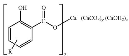
wherein R is an alkyl group derived from said isomerized alpha olefins and wherein y and z are independently whole or partial integers; and further wherein said overbased alkylated hydroxyaromatic carboxylate detergent has a TBN of greater than 250.
