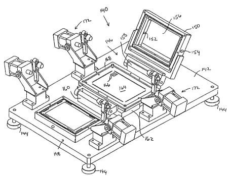
(57) Abstract: A device and method for distributing solid supports has a flow system (150), an attraction device (162), and a receiver (148). The flow system (150) is positioned over the attraction device (162) where particles are attracted into holes (166) in an attraction surface (164) using vacuum. The flow system (150) is removed and the attraction device (162) is positioned over the receiver (148) and the particles transferred to the receiver (148) by pressure and/or vacuum.
