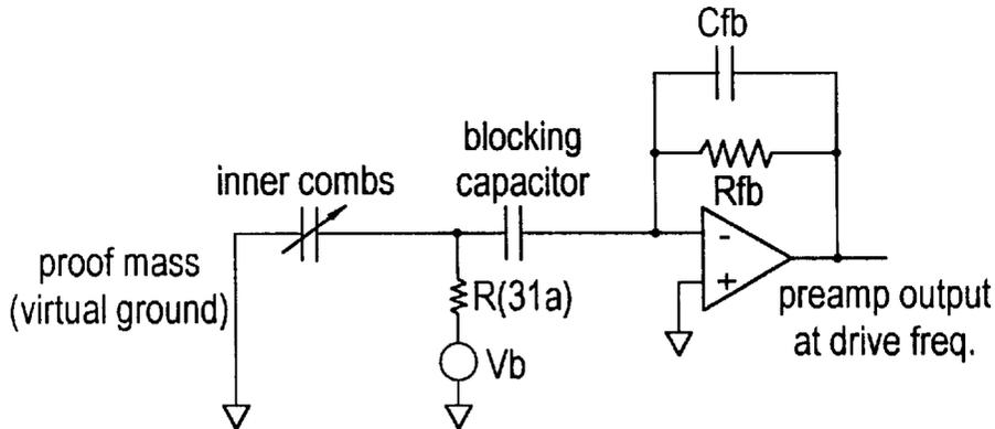
**Biasing motor sense combs with fixed voltage and blocking capacitor.**
