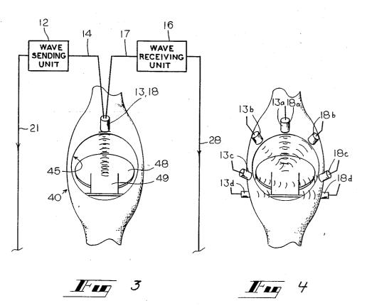
tion of check valve components without requiring physical inspection of the valve components nor requiring back flow of fluid.
