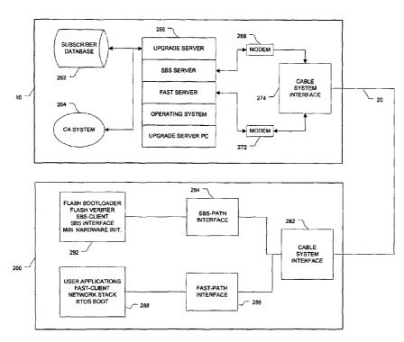
(57) Abstract: A system (10) and method (400) for downloading code or other data to a group of remote units (200) via a plurality of data paths (20). The data paths used for transmission may be selected based on the criticality of the code or data to the remote unit and the loss rate potential of each data path. The system and method may download the data using a carouselling technique (300).
