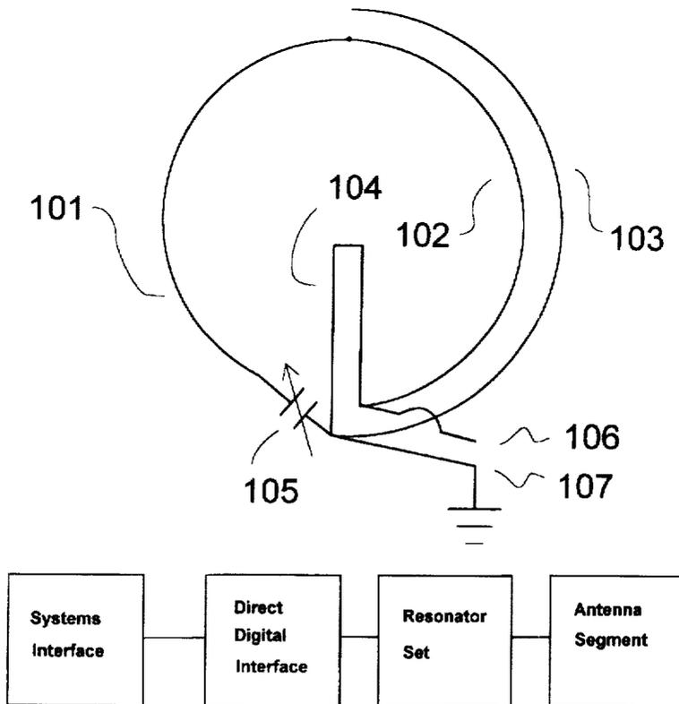
**Tunable Resonator Antenna Circuit System
