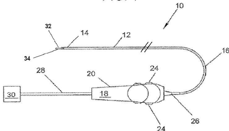
(57) Abstract: An imaging and treatment device comprises a catheter body, an imaging transducer, and an elongated member. The imaging transducer is disposed at a distal portion of the catheter body. A treatment element is disposed at a distal end of the elongated member, and the elongated member is movable within a lumen of the catheter body.
