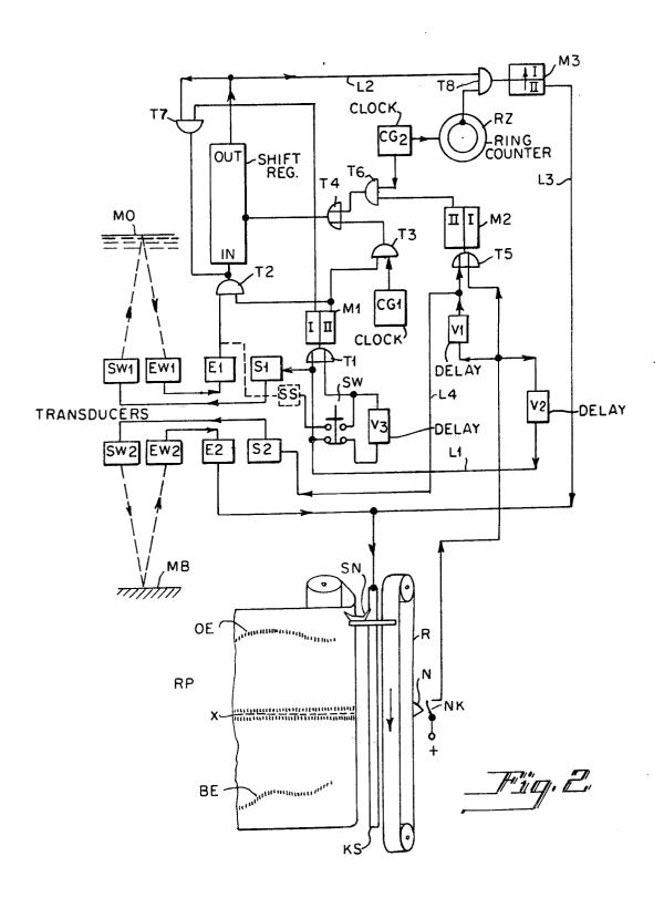
METHOD AND SYSTEM FOR THE POSITIONALLY CORRECT RECORDING OF TWO ECHO SIGNALS FROM RESPECTIVE ECHO SOUNDINGS TAKEN IN MUTUALLY OPPOSED SOUNDING DIRECTIONS
