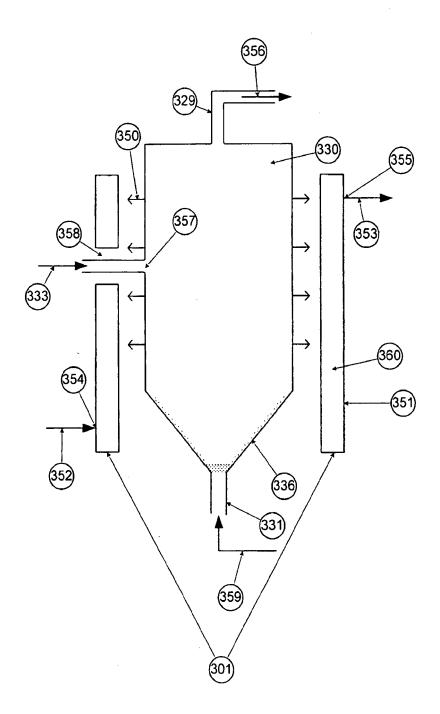
Fig 3. Schematic of the product separator with integrated heat recovery
