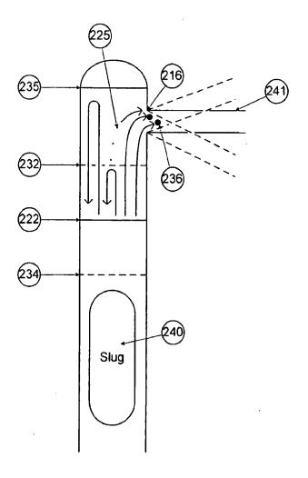
Fig 2b. Detail schematic of the granular particle removal mechanism
