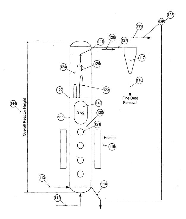
Fig 1. Typical Fluidized Bed Deposition Reactor
