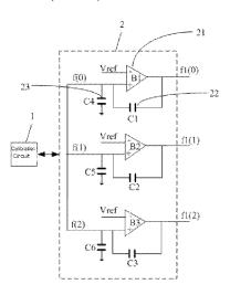
circuit calibrates the capacitance of the sensing capacitor to a capacitance that matches with the current frequency point.
