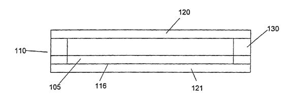
(57) Abstract: An encapsulation for an electrical device (105) is disclosed. The encapsulation comprises plastic substrates (120, 121) which are laminated onto the surface (116) of the electrical device (105). The use of laminated plastics is particularly useful for flexible electrical devices (105) such as organic LEDs.
