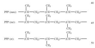
The triad tacticity (mm fraction) of the propylene copolymer can be determined from a <sup>13</sup>C-NMR spectrum of the propylene copolymer and the following formula:
