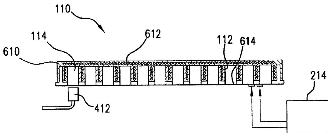
SECTION VIEW OF MICROTITER PLATE
