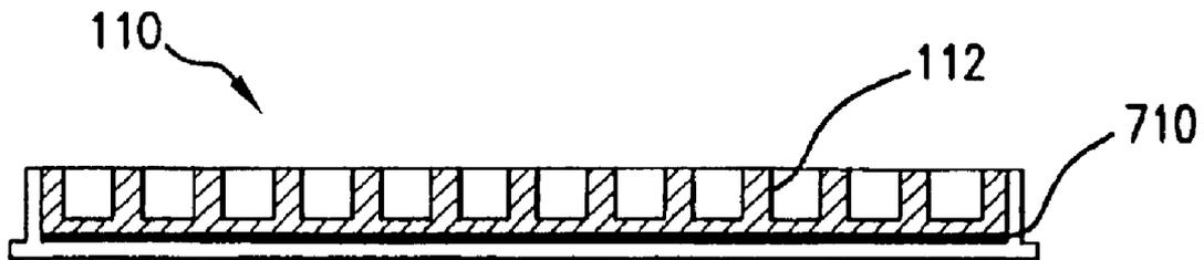
SECTION VIEW A-A' PLATE WITH INTEGRATED FERROUS PLATE FOR NON-CONTACT HEATING
