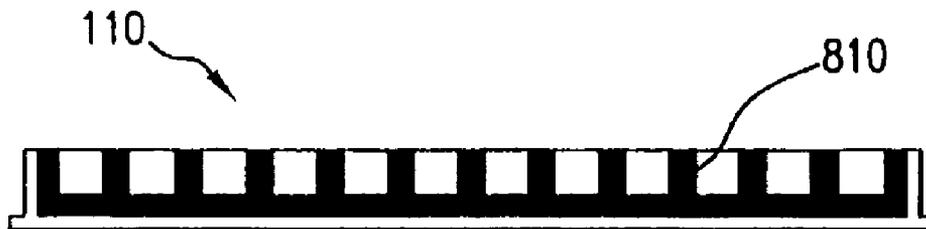
SECTION VIEW A-A' PLATE WITH FERROUS CONDUCTIVE MATERIAL FOR NON-CONTACT HEATING
