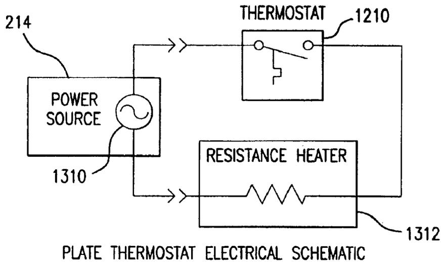
PLATE THERMOSTAT ELECTRICAL SCHEMATIC
