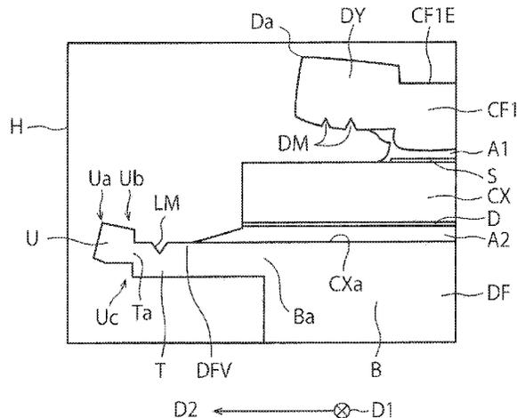
conductive connection member disposed between the first electrode on the semiconductor chip and a lower surface of the first clip frame, the first clip conductive connection member electrically connecting the first electrode of the semiconductor chip and the lower surface of the first clip frame; and a sealing resin for sealing the semiconductor chip, the die pad frame, the first clip frame, the first clip conductive connection member, and the conductive connection member for die pad.
