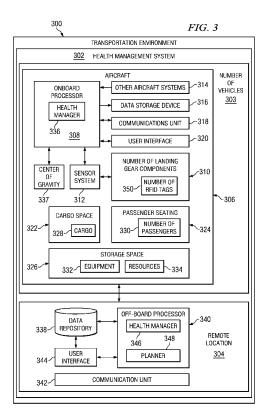
(57) Abstract: The different advantageous embodiments provide an apparatus comprising a number of landing gear components (310) for a vehicle, a number of systems (314), and a number of processor units (308). The number of systems is configured to generate data about the number of landing gear components and the vehicle. The number of processor units is configured to monitor the data and manage health of the number of landing gear components.
