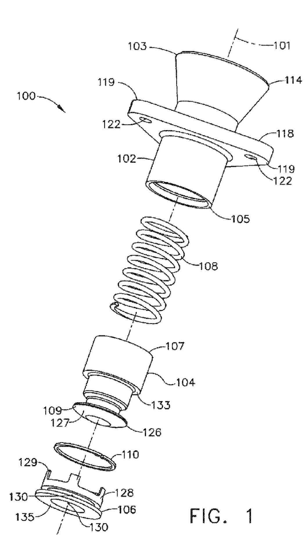
(57) Abstract: An assembly is provided with a housing, a guide sleeve, and a spring. The guide sleeve may be at least partially housed within the housing. The spring may be disposed to abut against the housing and the guide sleeve.
