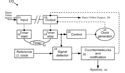
Output to input synchronization and signal detection
