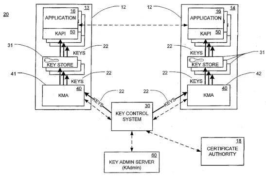
(57) **Abstract:** A system for automated cryptographic key management comprises a key control system, a key management agent system, and a key system application program interface. A method for automated cryptographic key management is also disclosed. The method comprises the automatic generation of cryptographic keys by the key control system and distribution of such keys by the key control system to the key management agent system.
