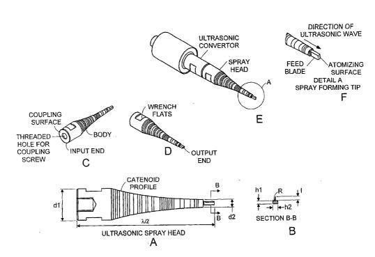
(57) Abstract: Disclosed is an ultrasonic spray coating system comprising an ultrasonic transducer with spray forming head, integrated fluid delivery device with air and liquid supply passage ways, support brackets and an ultrasonic power generator.
