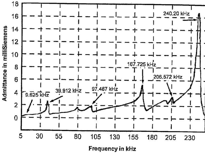
Sweep 5 kHz – 250 kHz, Air Load
