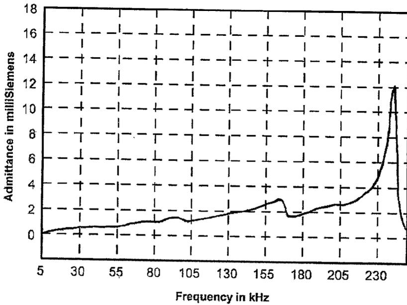
Sweep 5 kHz – 250 kHz, 'Mastoid' Load
