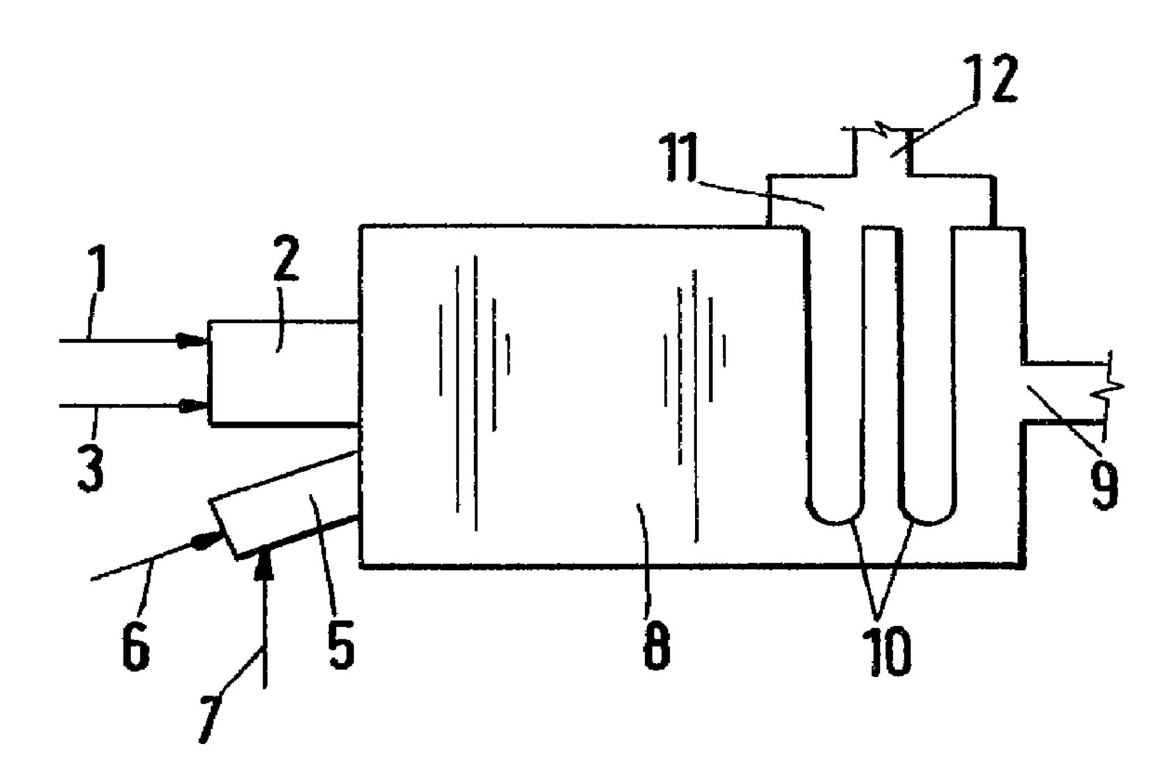
(57) The H<sub>2</sub>S-containing gas is combusted with oxygen in at least one burner, which discharges into a combustion chamber. The resulting mixed gases contain H<sub>2</sub>S, SO<sub>2</sub>, free hydrogen and elementary sulfur and are at temperatures of about 900 to 2000°C. At temperatures of about 900 to 2000°C at least part of the free hydrogen is removed from said mixed gases. The free hydrogen may be removed from the mixed gases, e.g., through membranes.
