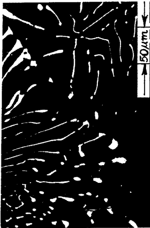
MC TYPE CARBIDES IN STEEL C11V FIG. 6
