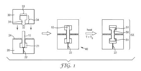
(57) Abstract: Fasteners for producing double blind joints where the fastener is not visible or accessible are provided. The fasteners comprise a shape memory polymer that may be used to fasten workpieces by heating the fasteners, inducing recovery of the original, permanent shape of the fasteners
