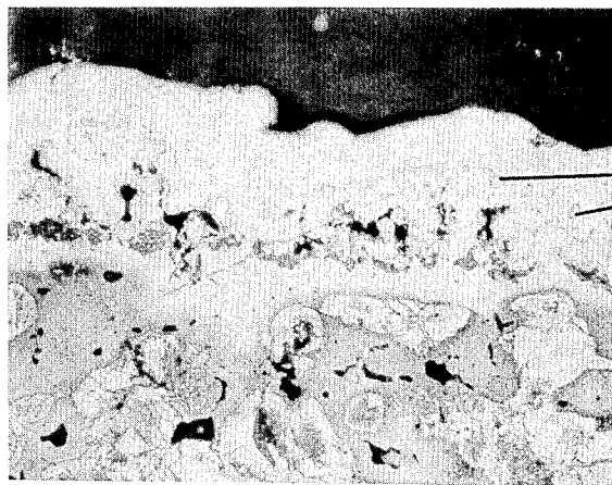
FIG. 10 SINTERED WC PARTICLES IN NICKEL MATRIX OF COATING
